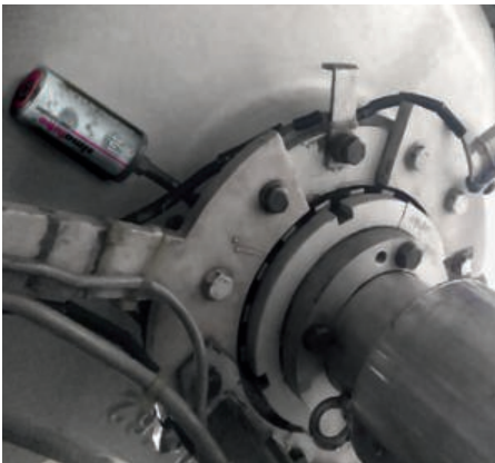
With the practical simalube accessories, it is possible to easily equip each lubrication point with a simalube dispenser.
